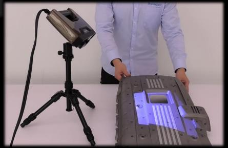
If scanning without a turntable, there should be at least a 30% overlap to ensure alignment.
