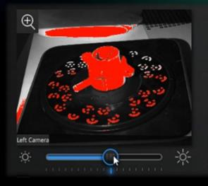
Avoid overexposure by reducing the brightness level
